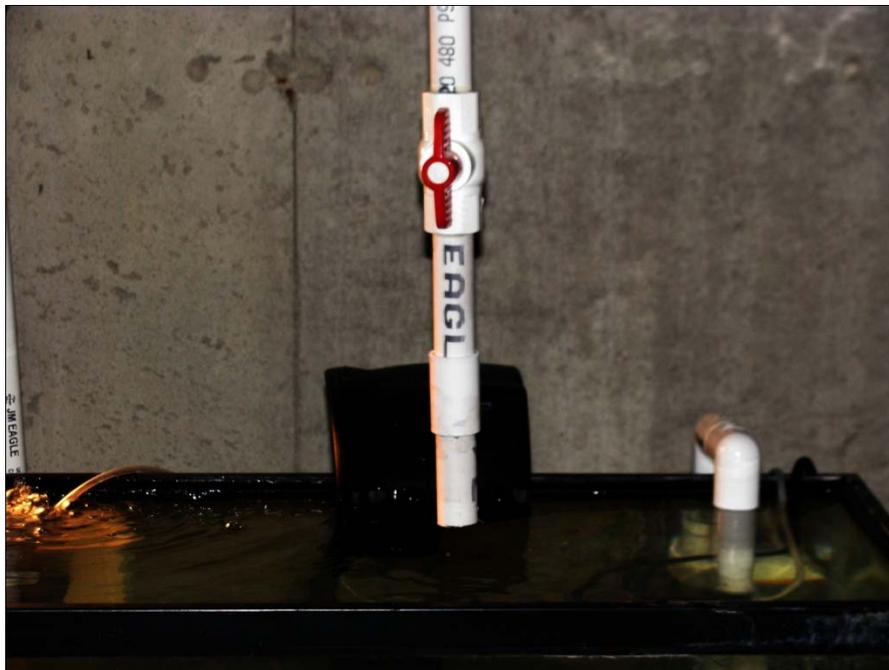
**Detail of fill pipe, along with cut-off valve**
